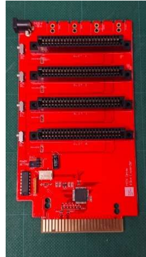
SLOT Expander with audio output function by Illegal function call
